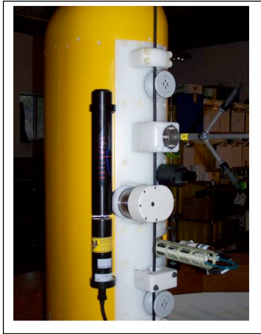
Figure P-8: Completed SUNA Installation
