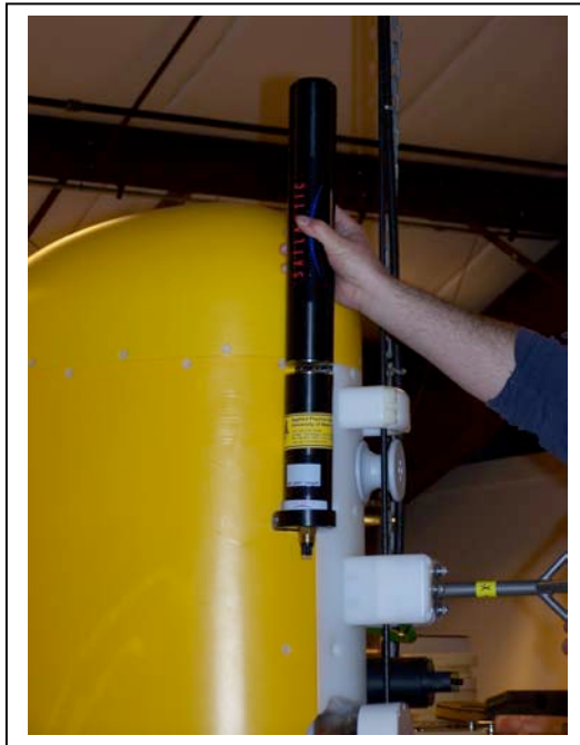
Figure P-3: Sliding the SUNA into the Sensor Brackets
