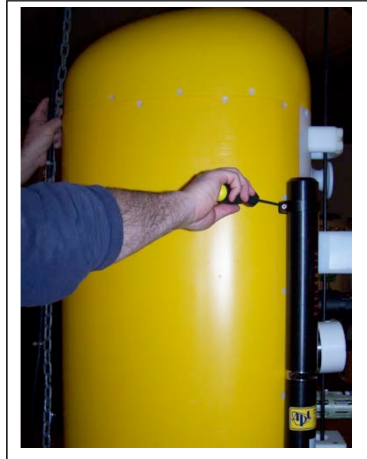
Figure P-4 and P-5: Tightening Bottom and Top Mounting Screws
